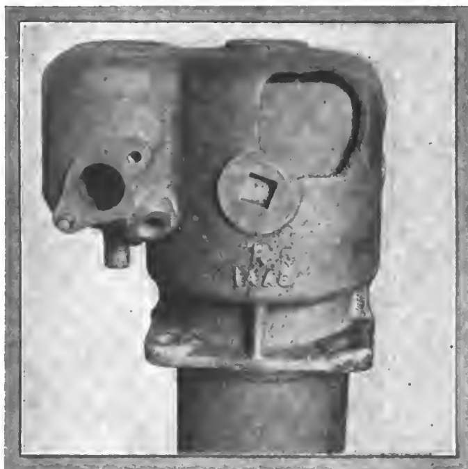
Fig. 4—Broken water jacket which can be welded by the oxy-acetylene process if the missing part is not lost
